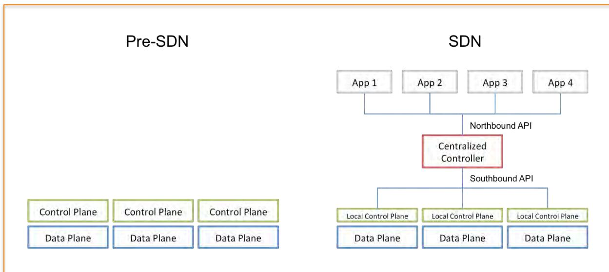
By centralizing certain key aspects such as routing configuration, path calculation, inventory tracking and network statistics, the centralized controller can become much more intelligent, and can optimize network traffic in a way that was not possible before.
