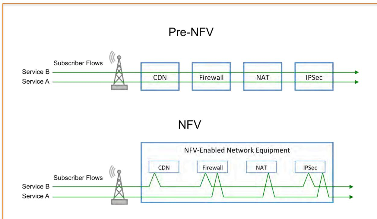
In today's networks, because many of these functions are standalone physical devices, the physical network connections are configured in
