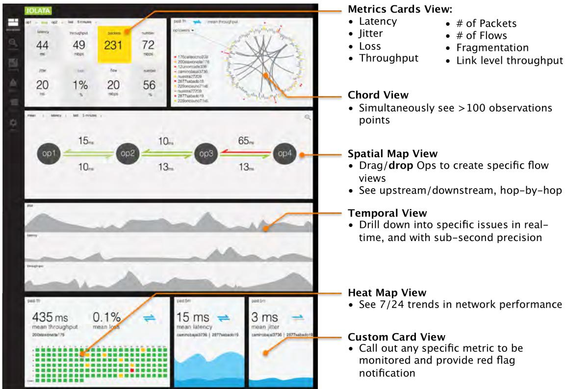
The Chord diagram (top right) provides a holistic view of up to 150 individual network locations or observation points, each OP represented by a “compass point” on the circumference of the chord. The Chord diagram shows qualitatively which parts of the network are over- or under-utilized.
